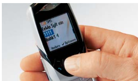
The Vitocom 100 receives your commands via SMS – and also informs you of faults.
